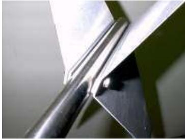
To install the tail boom, orient the boom with the longer fins pointing down and the hole in the boom lined up with the corresponding hole in the wind turbine housing. Insert the tail boom into the housing and when it is snugly seated with the holes aligned, secure with an M10 x 70 bolt, two flat washers (one on each side of the turbine housing) and an M10 nylock nut. Torque to 75 Nm (55 ft lbs). Put a drop of medium strength lock tight on each thread.
