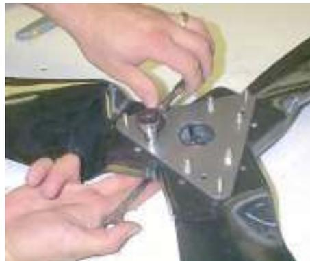
This is best accomplished by measuring the distance between the leading edge of one blade to the trailing edge point of the adjacent blade as shown in the following photographs and adjusting the blades until all three measurements are equal. The blade tips are contoured so take special care to use the same points on the tip for each measurement.
