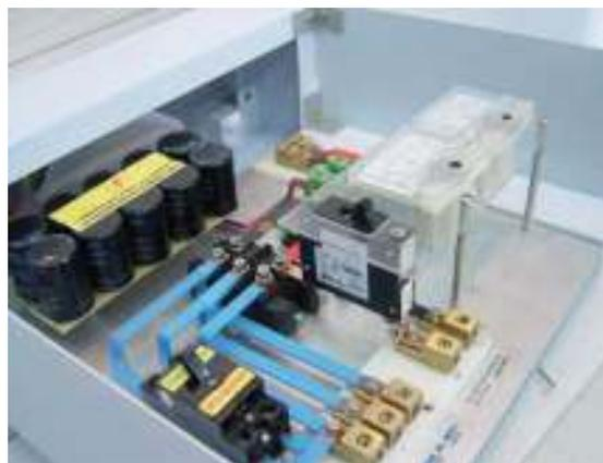
Once the test has been successfully completed connect the cables to the three terminals on the AC input side of the controller-rectifier. For a more detailed discussion regarding the wiring of the Commander refer to the section entitled 'Wiring the LAKOTA Commander' on pgs 29-30.
