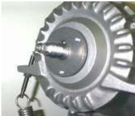
Place the aft hub plate onto the wind turbine shaft, ensuring that the large hole in the centre seats beyond the shoulder of the shaft and carefully aligning the three inner holes of the aft hub plate with the three holes on the hub torque ring. Fasten the aft hub plate to the hub torque ring using three M6 x 12 cap screws with a few drops of permanent (red or green sometimes provided in a small vial) thread
